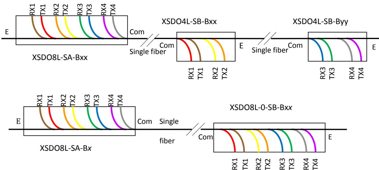
Figure 1 Multichannel single fiber connection examples
