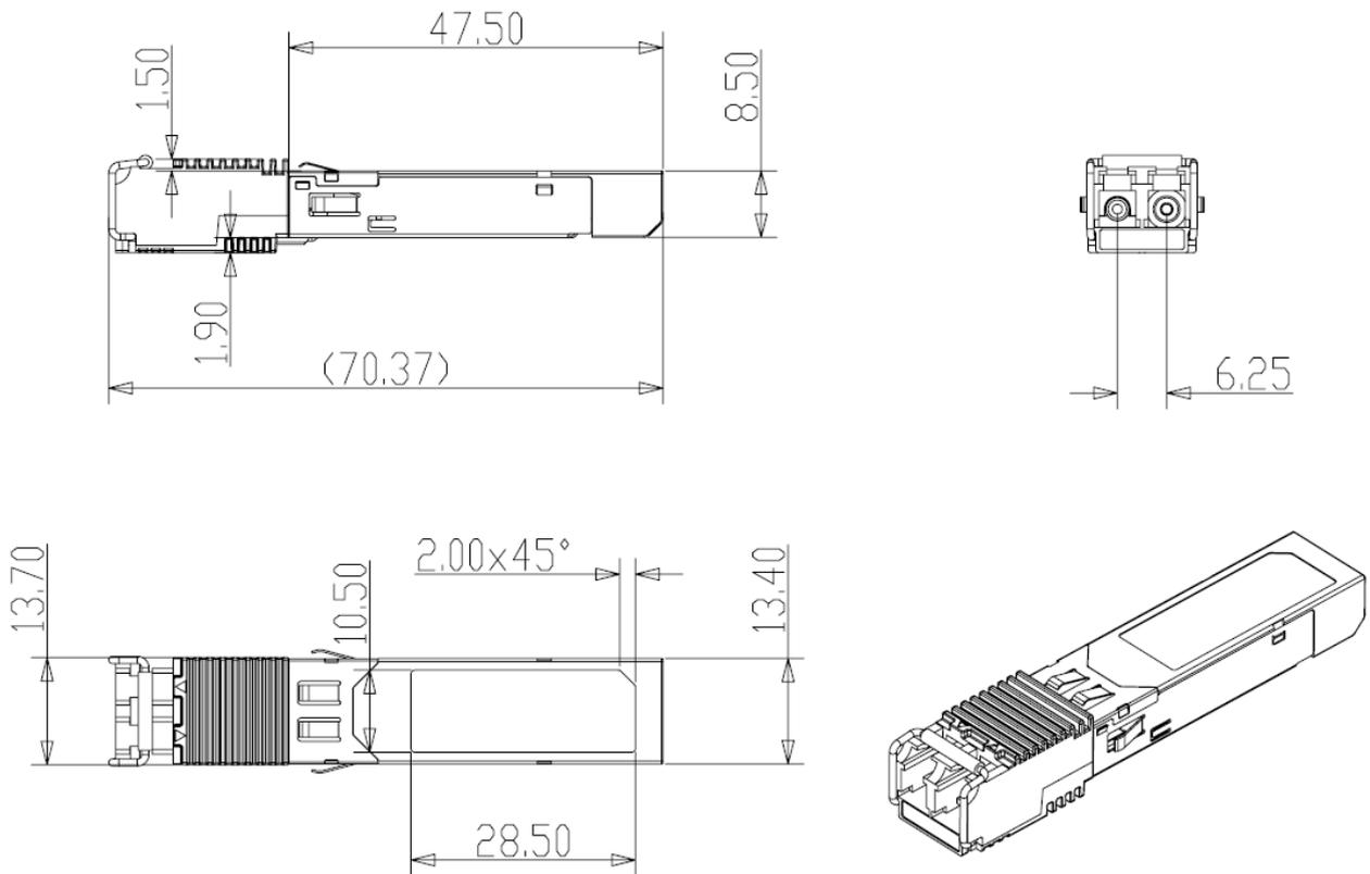
**Figure 5. Mechanical Specifications**
