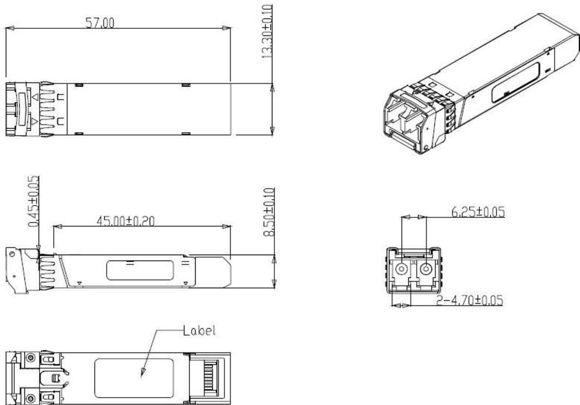
**Figure 5. Mechanical Specifications**
