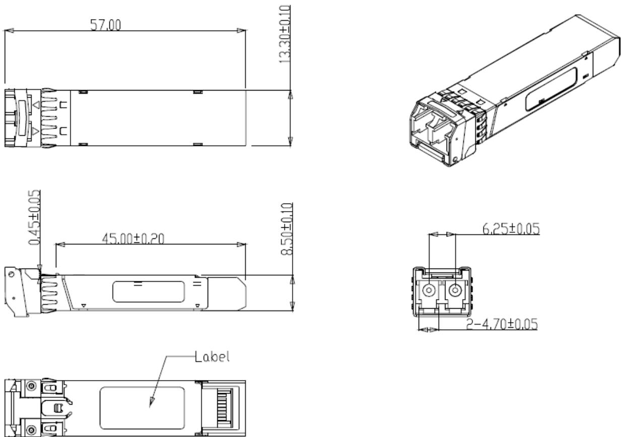
**Figure 5. Mechanical Specifications**
