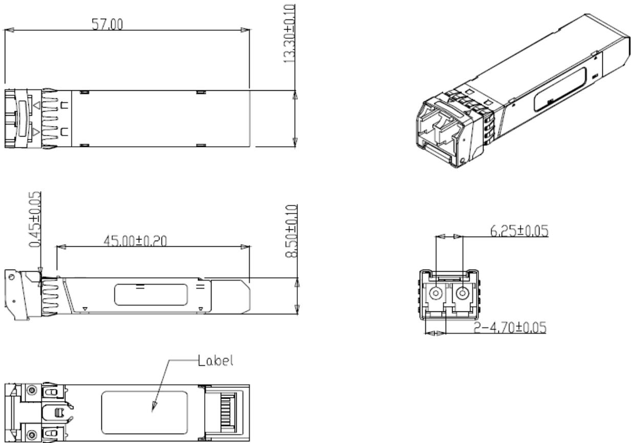
**Figure 5. Mechanical Specifications**
