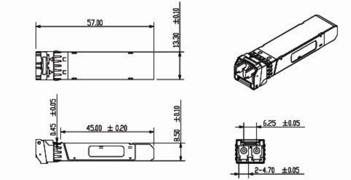
**Figure 4. Mechanical Specifications**
