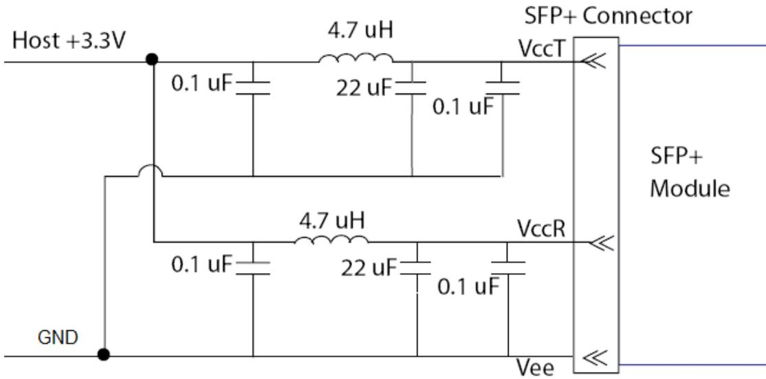
Figure 2. Host Board Power Supply Filters Circuit
