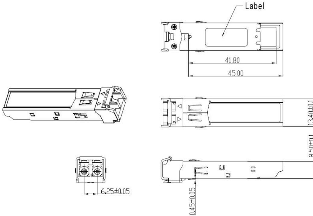
Figure 4. Mechanical Specifications
