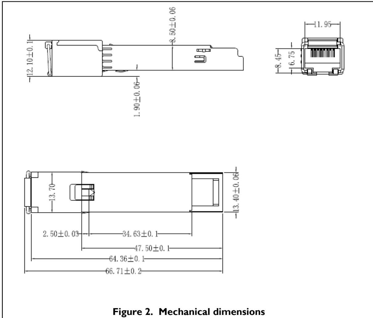
**Figure 2. Mechanical dimensions**
