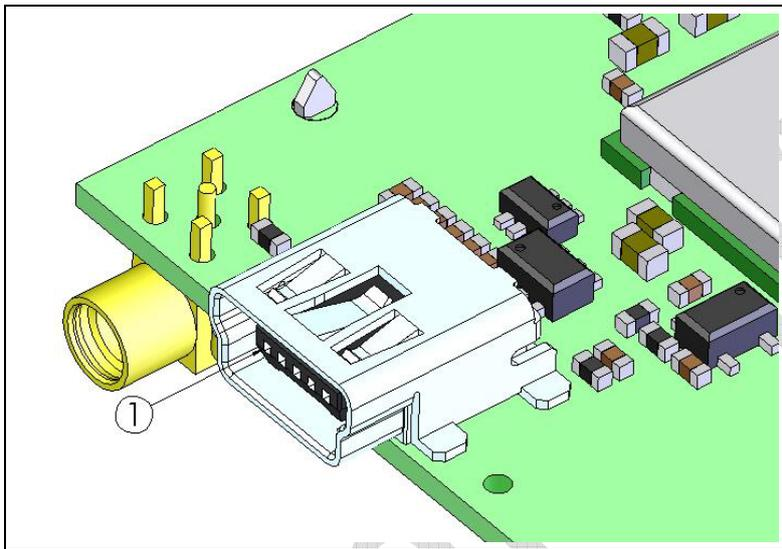
**Figure 6: Mini-B USB connector**
