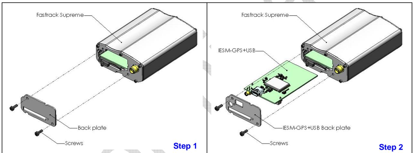
Figure 9: IESM-GPS+USB Mounting
