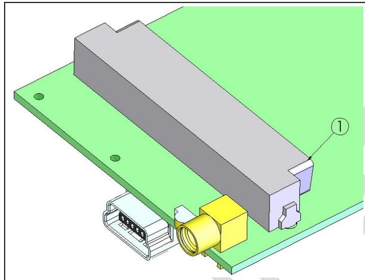
**Figure 7: IESM 50-pin connector**
