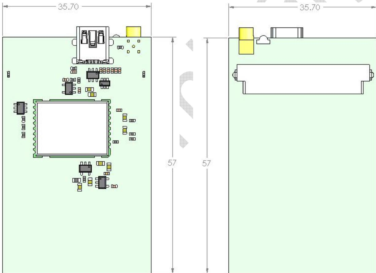
Figure 8: IESM-GPS+USB Dimensions
