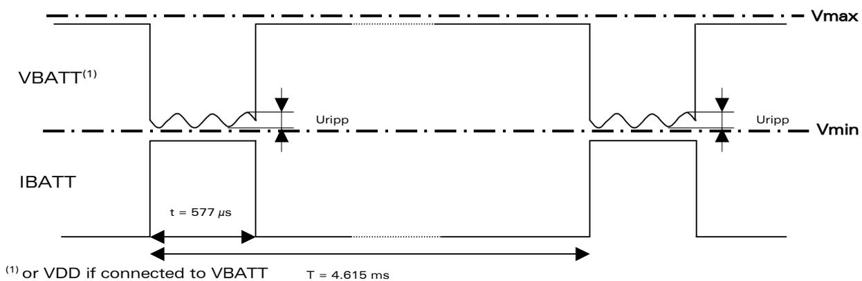
**Figure 2: Typical power supply voltage in GSM mode**
