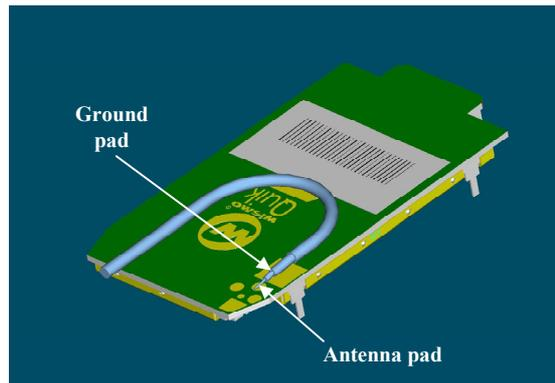
Figure 7: Antenna connection
