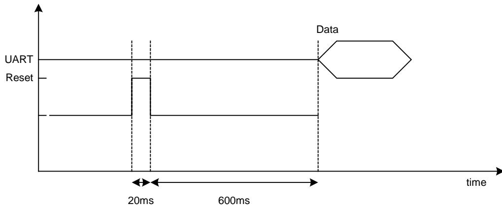
Reset signal with the configuration: AT+WBTCNF=0,0,20,600
