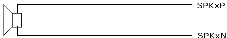
Figure 4 : SPK outputs (differential connection)
