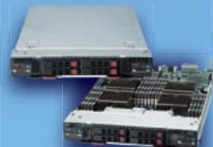
**TwinBlade w/ Two 2.5" Hot-plug Drive Bays per DP node**
