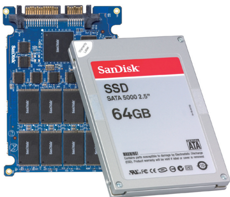
Figure 1: Solid State Components Inside a SSD
