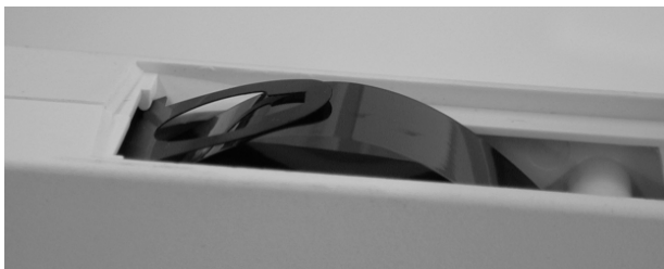
Figure 5-10 Examples of Tape Cartridge Loop Problems in DLTape IV or Earlier Versions
