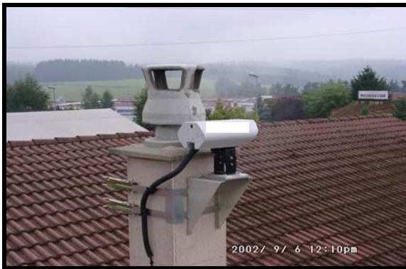
Figure 10: Wall Mounting (using JMP and JMB)
