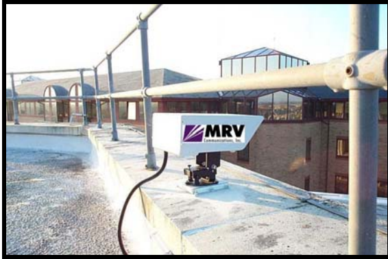
Figure 9: Parapet/Ledge Mounting (using JMP only)
