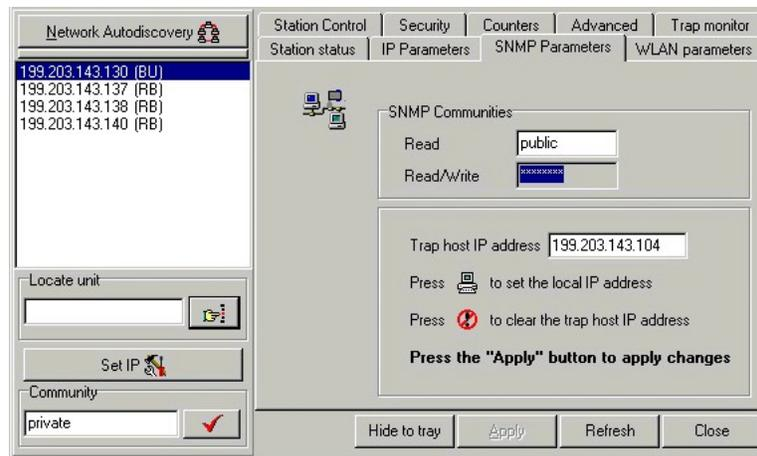
**Figure 3-10. SNMP Parameters Tab**
