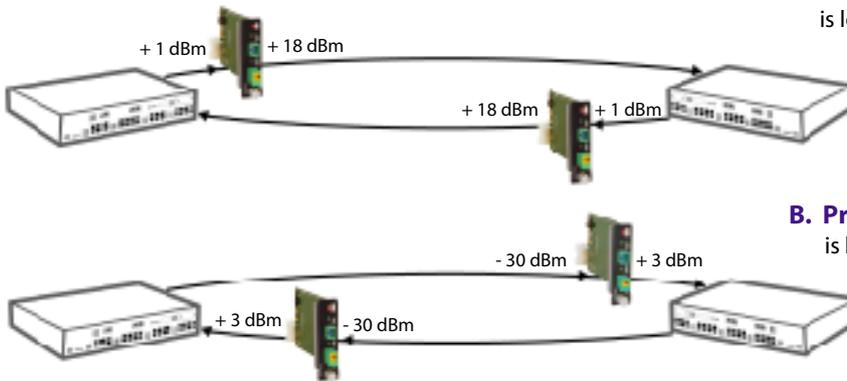
**A. Booster Amplifier** – The optical amplifier is located close to the signal source.
