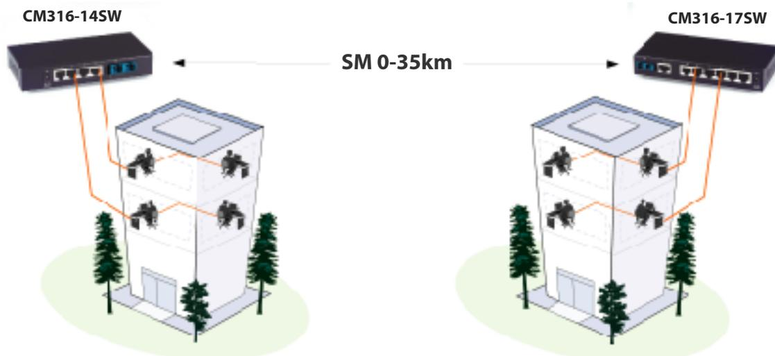
When configured with a DSC Multimode optic transceiver, the FX port can achieve link distances of up to 2 km. With a DSC Singlemode optic transceiver, FX port link distances can reach up to 35 km.
