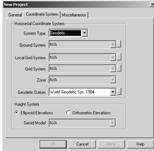
**Figure 3.3.** New Project Dialog Box — Coordinate System Tab
