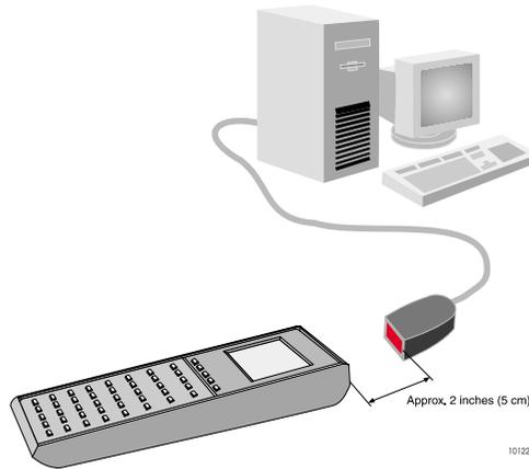
**Figure 4.6.** Setup for Transferring HP-48 Handheld D-Files
