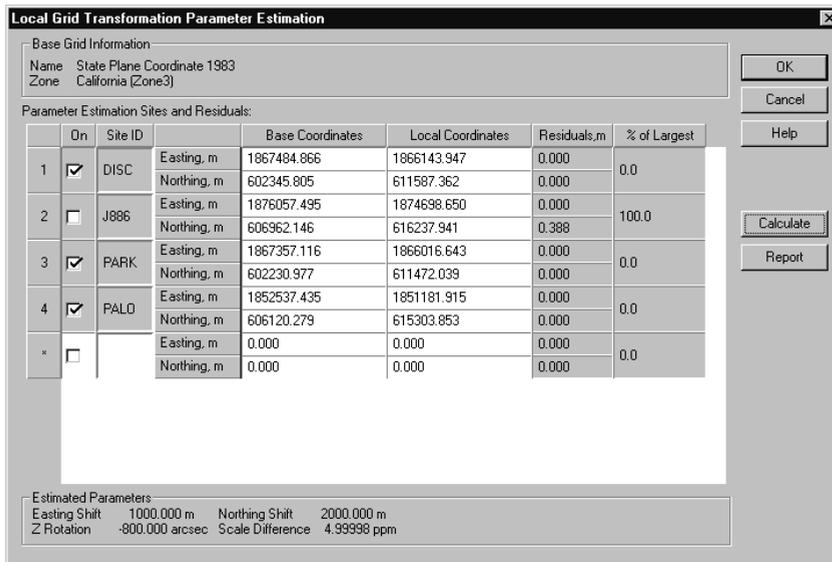
**Figure 9.9.** Local Grid Transformation with Estimated Parameters
