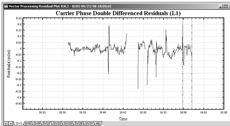
**Figure 5.12.** Vector Processing Residual Plot
