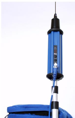
**Figura 3.18.** Radio Rover PDL Pacific Crest con Antena
