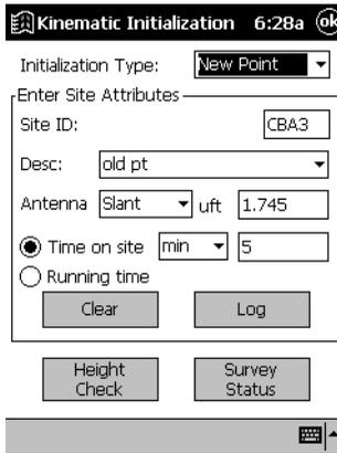
**Figure 4.22** Kinematic Initialization Screen
