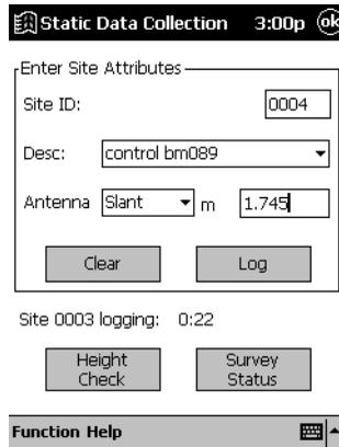
**Figure 4.5** Static Data Collection Screen
