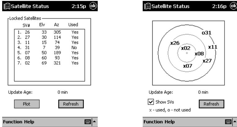
**Figure 3.28** Satellite Status Screens - Table (left) and Plot (right)
