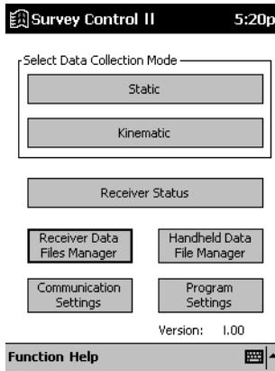
**Figure 2.6** Survey Control II Main Screen
