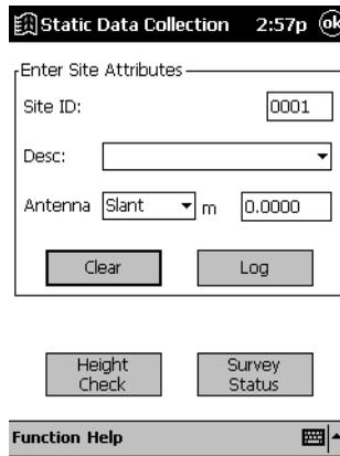
**Figure 3.14** Static Data Collection Screen
