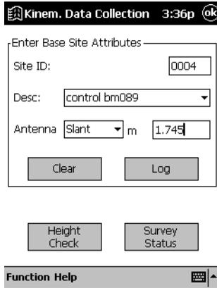
**Figure 2.18** Base Kinem. Data Collection Screen
