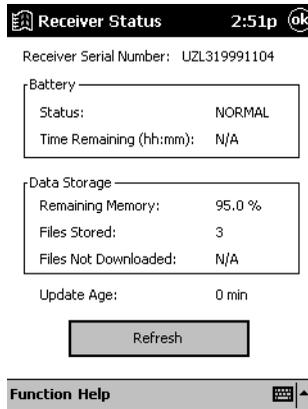
**Figure 2.9** GPS Receiver Status Screen
