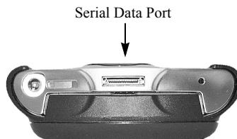
**Figure 2.26** Handheld Serial Data Port
