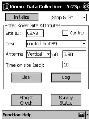
**Figure 2.19** Rover Kinem. Data Collection Screen
