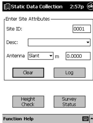
**Figure 2.17** Static Data Collection Screen
