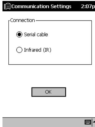
**Figure 3.4** Communication Settings Screen- Serial for Z-Xtreme, IR for Locus
