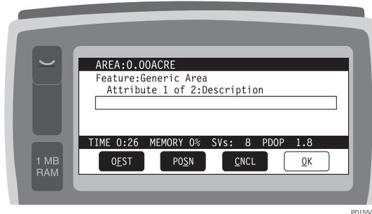
**Figure 3.68:** Feature Logging Screen, Real-Time Area Calculation
