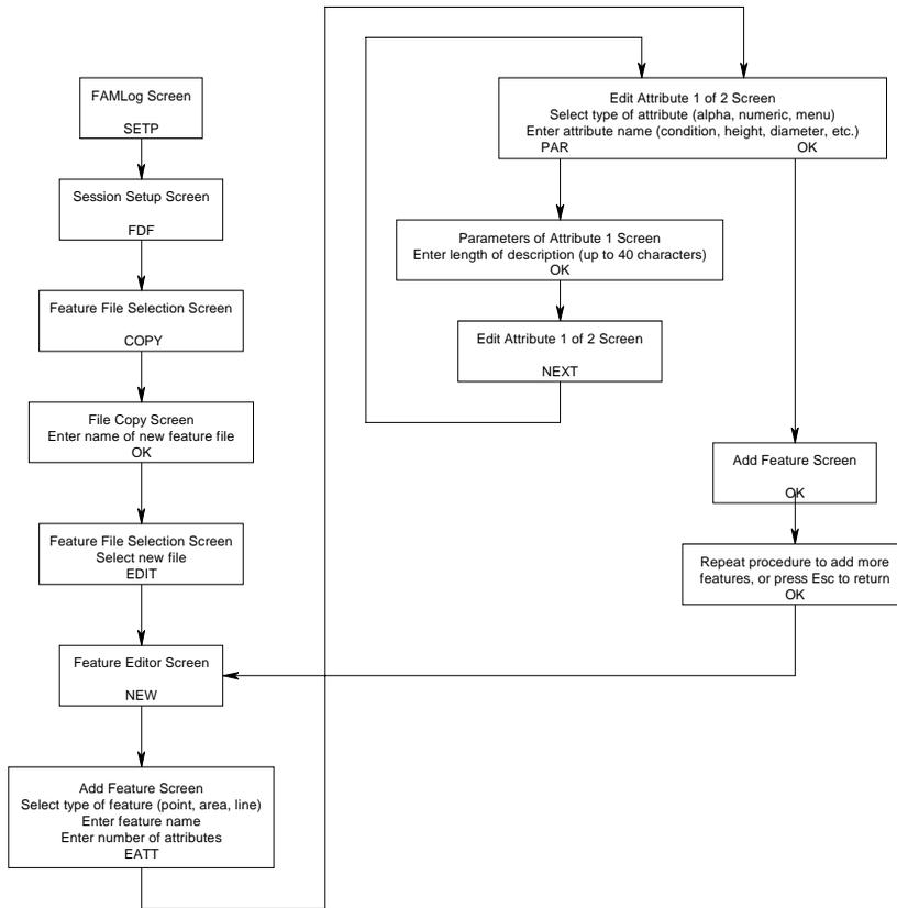
**Figure 3.42:** Screens and Process for Adding Features
