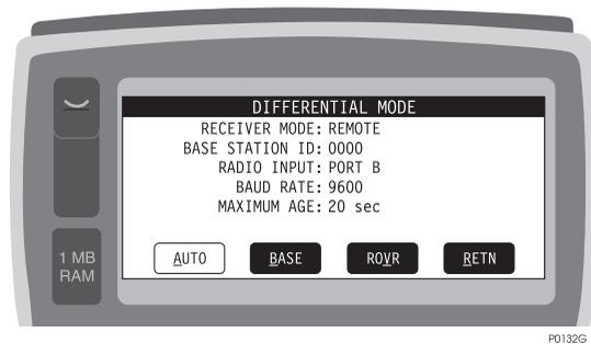
**Figure 4.38:** Differential Mode Status Screen (MODE) - 2
