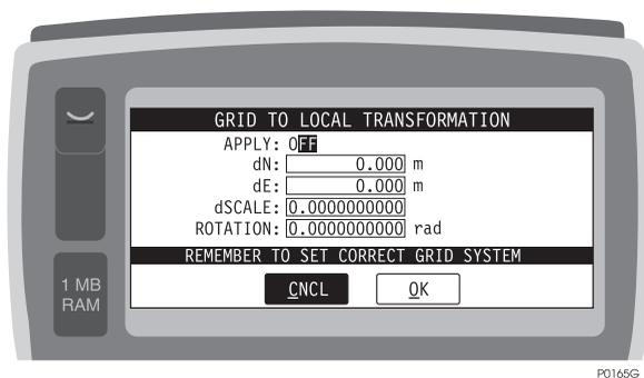
**Figure 3.88:** Grid to Local Transformation Screen
