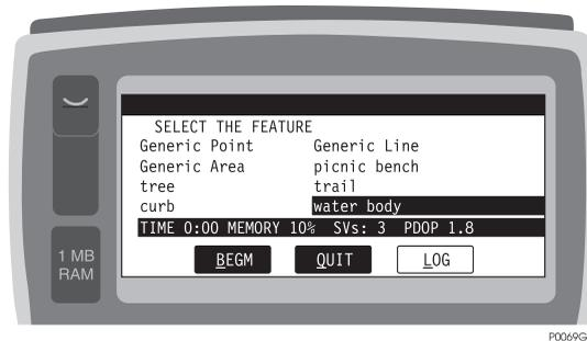
**Figure 3.11:** Selecting First Feature - Water Body
