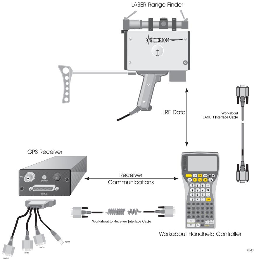
**Figure 3.35:** Configuration with LRF
