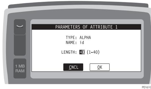
**Figure 4.58:** Parameters of Attribute Screen (PAR) - Alphanumerics
