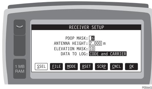
**Figure 4.32:** Receiver Setup Screen (RCVR)
