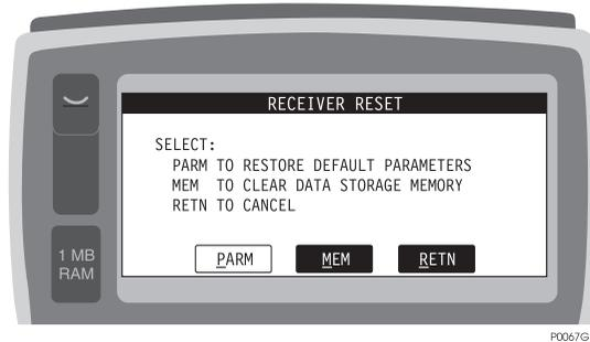
**Figure 3.8:** Receiver Reset Screen
