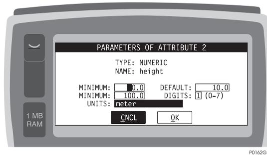
**Figure 4.59:** Parameters of Attribute Screen (PAR)
