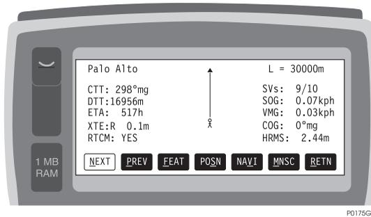
**Figure 4.16:** Vertical Line Navigation Status Screen (LINE)
