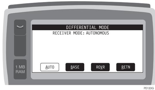
**Figure 4.37:** Differential Mode Status Screen (MODE) - 1
