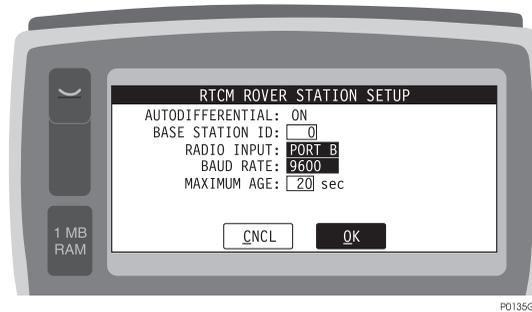
**Figure 3.59:** RTCM Rover Station Setup Screen
