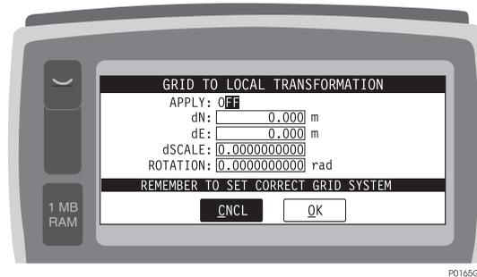
**Figure 4.29:** Grid to Local Transformation Screen (LOCL)
