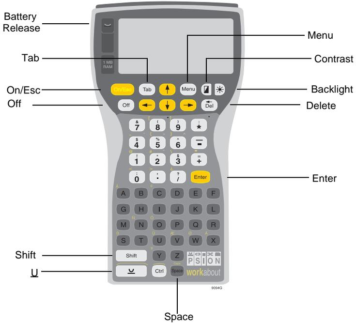
**Figure 1.2:** Workabout Handheld Controller
