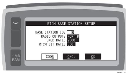
**Figure 4.41:** RTCM Base Station Setup Screen (BASE)
