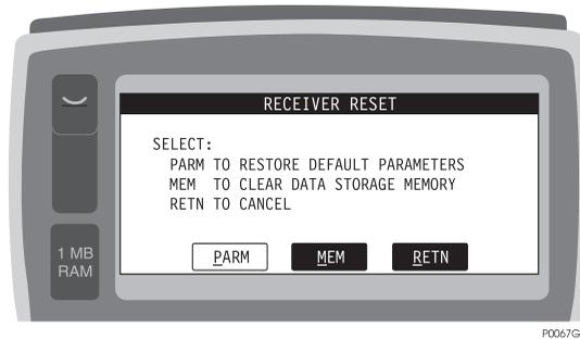
**Figure 4.36:** Receiver Reset Screen (RSET)
