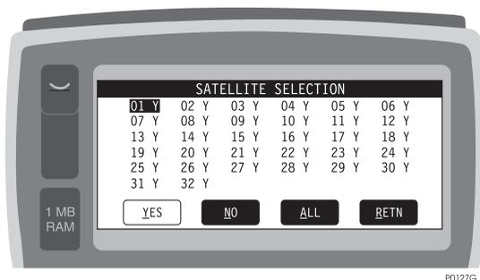
**Figure 4.33:** Satellite Selection Screen (SSEL)
