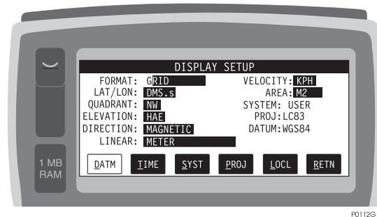
**Figure 4.18:** Display Setup Screen (DSST), Grid
