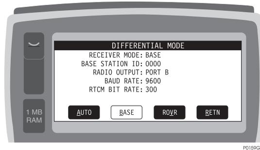
**Figure 4.39:** Differential Mode Status Screen (MODE) - 3
