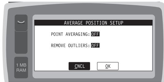
**Figure 4.51:** Average Position Setup Screen (AVST)
