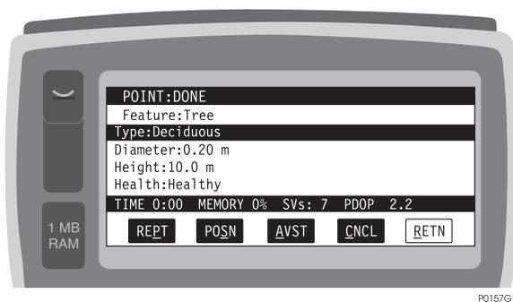
**Figure 4.45:** Logging Status Screen - Point (LOG)
