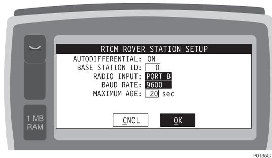
**Figure 4.40:** RTCM Rover Station Screen (ROVR)
