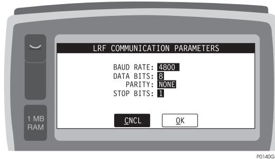
**Figure 4.49:** LRF Communications Parameters Screen (LCOM)
