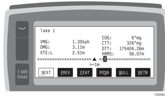
**Figure 4.14:** Horizontal Line Navigation Screen (NAVI)
