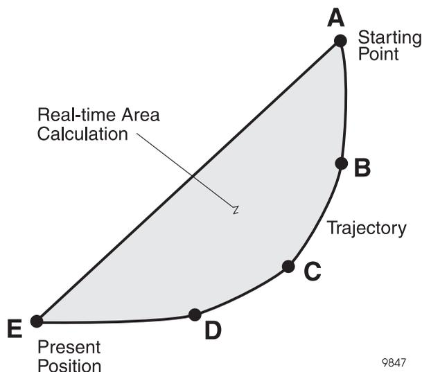
**Figure 3.63:** Automatic Area Calculation - RTCM Mode Only
