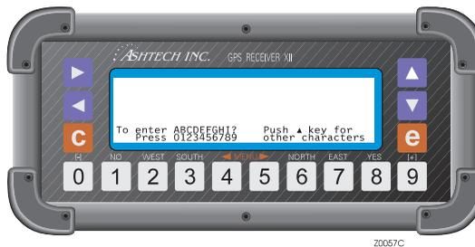
**Figure D.3:** Screen 9, Data Entry Mode
