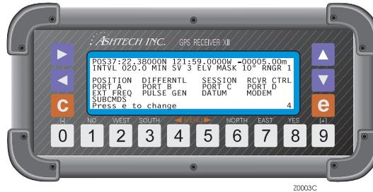
Figure 3.1: Screen 4, Data Entry Mode Screen
