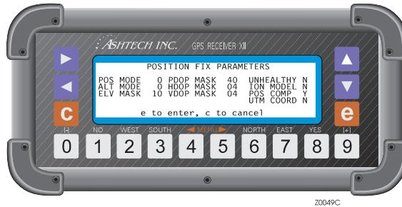
**Figure 4.7:** Position Fix Parameters Screen
