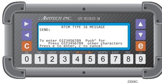
**Figure 3.7:** RTCM Type 16 "Send Message" Screen
