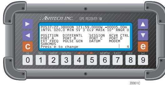
**Figure D.1:** Screen 4, Mode Control
