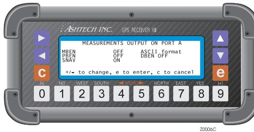
**Figure 5.3:** Measurement Output on Port A
