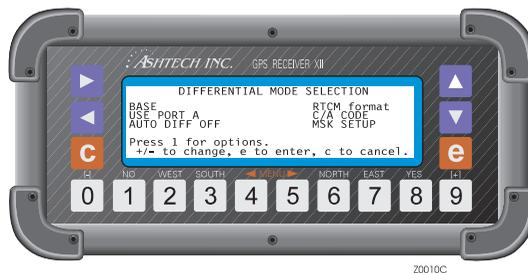
**Figure 3.9:** Differential Mode Selection Screen
