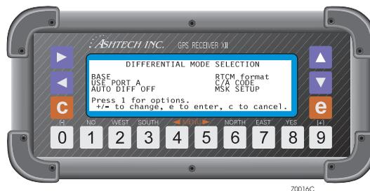
Figure 3.2: Screen 4, Differential Mode Screen
