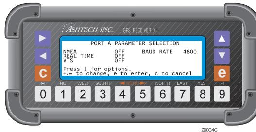
**Figure 5.5:** Screen 4, Port A Parameter Selection
