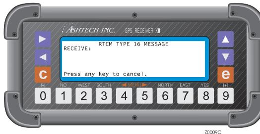
**Figure 3.8:** RTCM Type 16 "Receive Message" Screen
