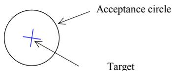
When you enter the acceptance circle of a target, the User Interface informs you of this event by displaying the "OK" message on the screen. The "OK" message will remain visible on the screen throughout the computing & logging phase as long as you stay within the limits of the circle.
