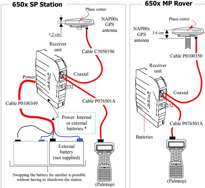
\*: Use either two camcorder-type batteries (not provided with station), or an external battery attached to the **Power** connector (located at the rear of the unit), using the cable provided (P0100349). In that case, make sure the CompactPro battery compartment is empty.
