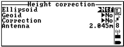
The ellipsoid used, as well the current value of antenna height above the ground are recalled on this screen. As in the planimetry function, you can only view the characteristics of the ellipsoid. You can however change the antenna height if necessary
