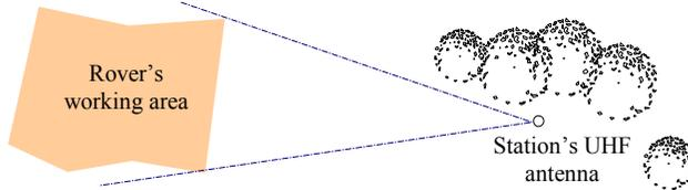
Note however that compared to optical systems for example, mutual visibility is not required. The presence of obstructions between UHF antenna and working area will admittedly cause the UHF signal to be somewhat attenuated, but in no case will it make the system unusable.
