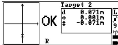
When the antenna position is within the acceptance circle (see definition in page 5-16), the **OK** message appears allowing you to log your current position.
