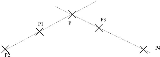
The system will determine the altitude of P by averaging the two extra or interpolated values obtained along straight lines P1P2 and P3P4, these two values being determined in the same way as in linear offset.
