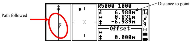
When the distance to the point becomes less than 5 m, the screen changes giving a magnified view of the area around the point ( $\pm 5$  m along each axis).
