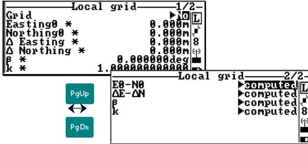
10. On screen 2/2, choose the grid computation options. The usual choice for all parameters is “Computed”. In this way, it is the barycenter of the working area (resulting from the selected reference points) that will be used as the origin (E0-N0) of the local grid. If you choose “Non-computed” for some of these parameters, then they will be fixed to their current values shown on screen 1/2.
