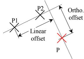
4. Select screen 2/3 and check to see if the resulting coordinates for the new point are consistent (no changes allowed on screen 2/3). Screen examples:
