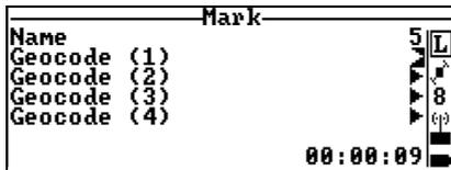
4. At the end of the event, press **F3**. A marker is created. On the screen, the time counter disappears and the marker name is incremented by one (for next marking operation).
