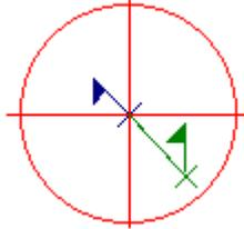
B. Target point whose solution is located outside the acceptable deviation limit (vertical flag and segment in red):
