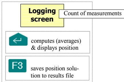
In point logging (scenario No. 1), note that the check stage may be bypassed by pressing **F3** directly. This enables computing and saving the position in a single operation.
