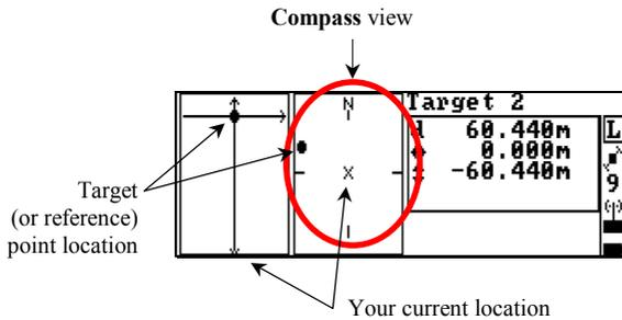
The direction to follow is given on the compass view (The North direction can be read on the rod's compass).
