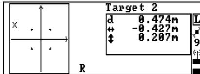
When the distance to the point becomes less than 0.15 m, the view can be magnified again ( $\pm 0.15$  m along each axis) by pressing the **PgDn** key. To come back to the  $\pm 0.5$  m view, press the **PgUp** key.
