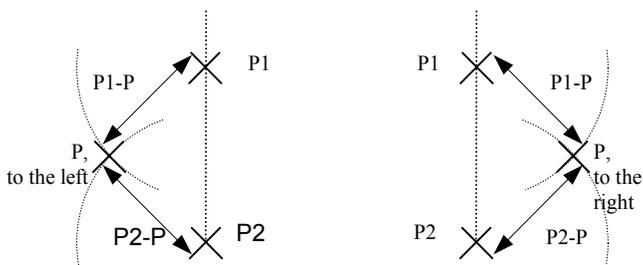
All computed distances are horizontal. The system will determine the altitude of P through linear interpolation along the P1P2 straight line (see page 5-20).
