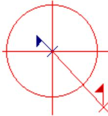
C. 3D target point whose solution is located outside the acceptable deviation limit due to the vertical component of the deviation (vertical flag and segment in red although they remain within the circle):
