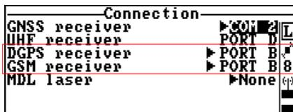
Port used on CompactPro to communicate with the GSM. The upper line indicates the port used to acquire the data from the GSM. Same as previously regarding the choice of port D for this connection
