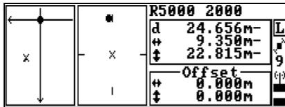
1. Press the T key (« T » for transverse) and type in the transverse deviation displayed in the upper-right frame:
