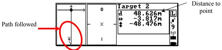
When the distance to the point becomes less than 5 m, the screen changes giving a magnified view of the area around the point ( $\pm 5$  m along each axis).
