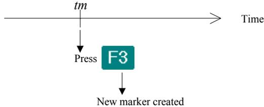
For example, this type of marker will allow 3S Pack to compute a position solution for that very particular moment in the recording.
