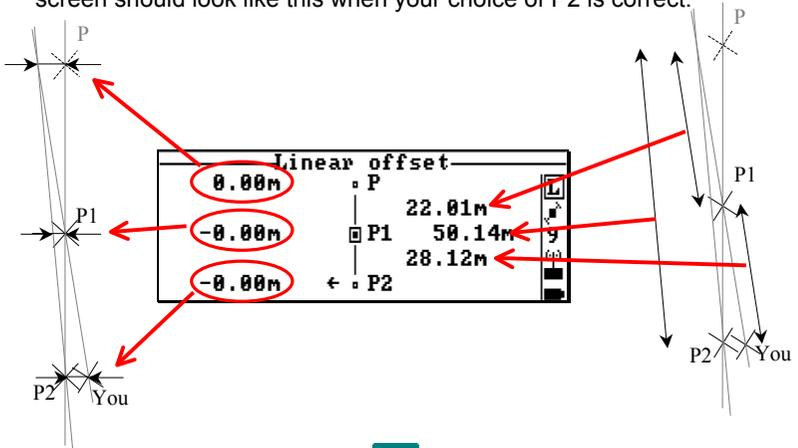
6. Select P2 on the screen. Press **F3** to compute and save the point position. Stay still until the message disappears.
