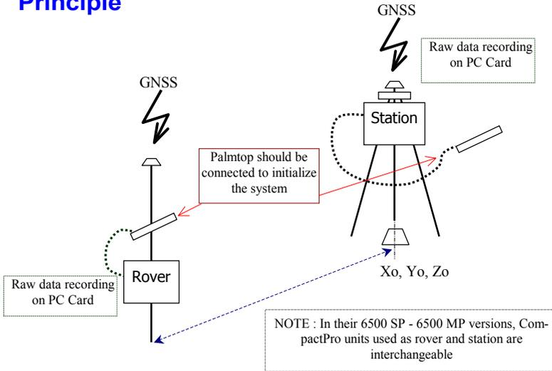
The palmtop allows you to set the recording rate and define the antenna height. It is also used to program automatic recording sessions, if you wish to use this function.
