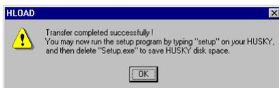
5. As prompted in this box, type “setup” and press
