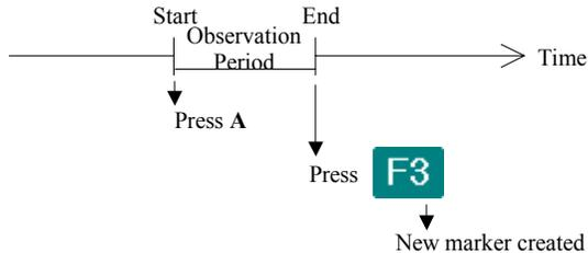
For example, this type of marker will allow 3S Pack to compute an averaged position solution over this observation period.
