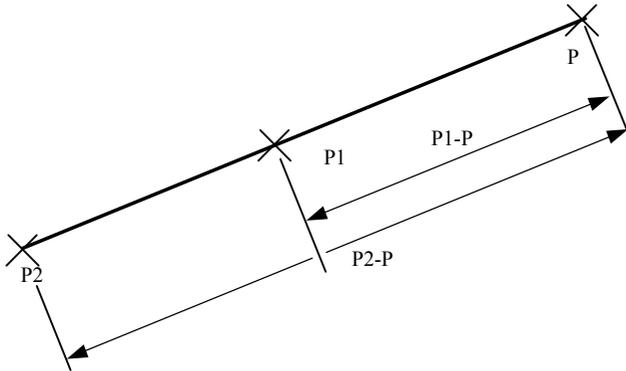
All computed distances are horizontal. The system will determine the altitude of P by interpolating the altitudes of P1 and P2 (see page 5-19).
