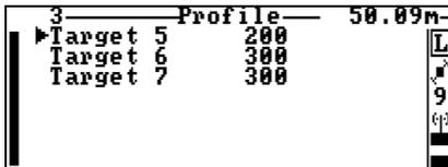
4. After selecting a point in the profile, press the
