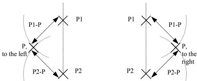
After measuring —with other means— the distances separating P1 and P2 from P, you will enter successively each of these distances when logging these points. You will also have to indicate on which side of the oriented segment P2P1 the P point is located (right or left).
