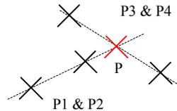
(You could also specify two points to define one straight line, and 1 point + 1 azimuth to define the other).
