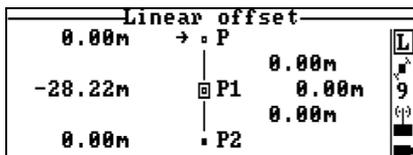
5. Walk in order to find a point P2 in the direction of the P1-P straight line where you will be able to compute a solution for that point. P2 will be aligned with the other two points when the indications on the left-hand part of the screen are all "0.0". The screen should look like this when your choice of P2 is correct:
