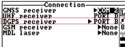
Port used on CompactPro unit to communicate with external DGPS receiver (B in general, possibly D if there was no built-in U-LINK receiver inside the Compact-Pro unit)
