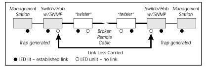
**IMPORTANT:** When connecting a "twister" media converter with LLCF enabled to an auto-negotiating device, force both sides of the configuration to either 10 or 100Mbps full or half duplex. This allows the interface media converter to immediately see link pulses and start passing data. Topology Solutions
