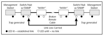
**IMPORTANT:** When connecting a "twister" media converter with LLCF enabled to an auto-negotiating device, force both sides of the configuration to either 10 or 100Mbps full or half duplex. This allows the media converter to immediately see link pulses and start passing data.
