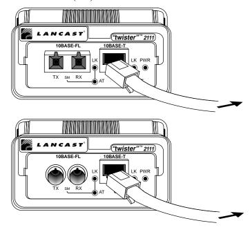
**Fiber Optic Connections** (2111-13, 2111-15, 2111-16, 2111-18). These "twister" models support 10BASE-FL segments via ST, SMA or SC connectors.
