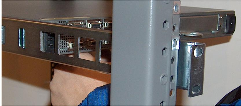
**Step 6.** Attach the rails to the rack, both sides as shown in Figure 4-8.
