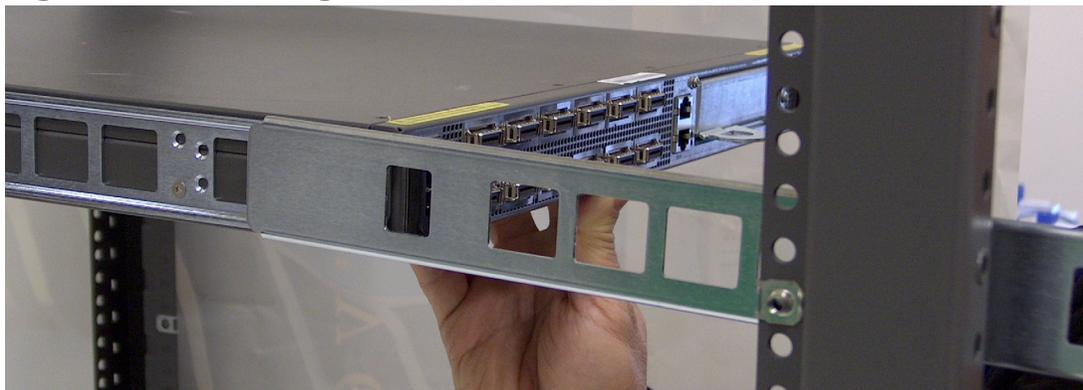
**Figure 4-7 Fit Sliding Rail to Rack**
