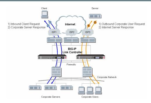
The BIG-IP Link Controller uses sophisticated monitors to detect errors across an entire link to provide end-to-end, reliable WAN connectivity. It monitors the health and availability of each connection, detecting outages to a link or ISP. In the event of a failure, traffic is transparently directed across other available links so end users stay connected.
