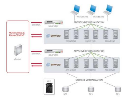
knows when virtual machines or entire data centers are overloaded or unavailable and reroutes traffic accordingly. With its in-built intelligence, BIG-IP can respond to fluctuating traffic loads without the need for manual intervention.
