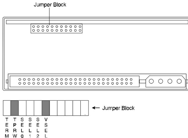
If you have a table top unit, you must set the VSEL switch on the back of the unit to the PC position (refer to Figure 2).
