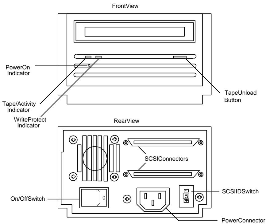
**Figure 1-2 Revised Version TLZ07-DA Tabletop Tape Drive**
