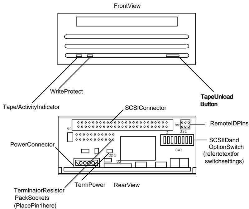
**Figure 1-4 Revised Version TLZ07-AA/-BA Tape Drive**
