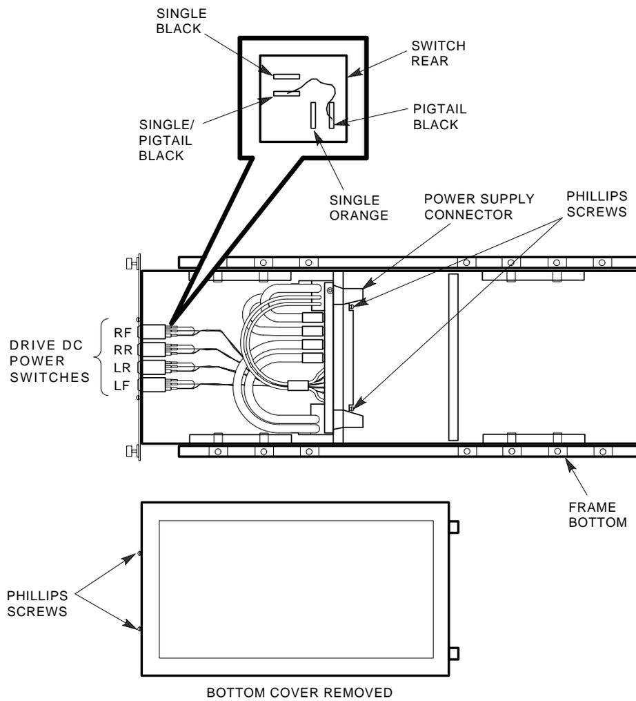
**Install the new drive dc power switch.**
