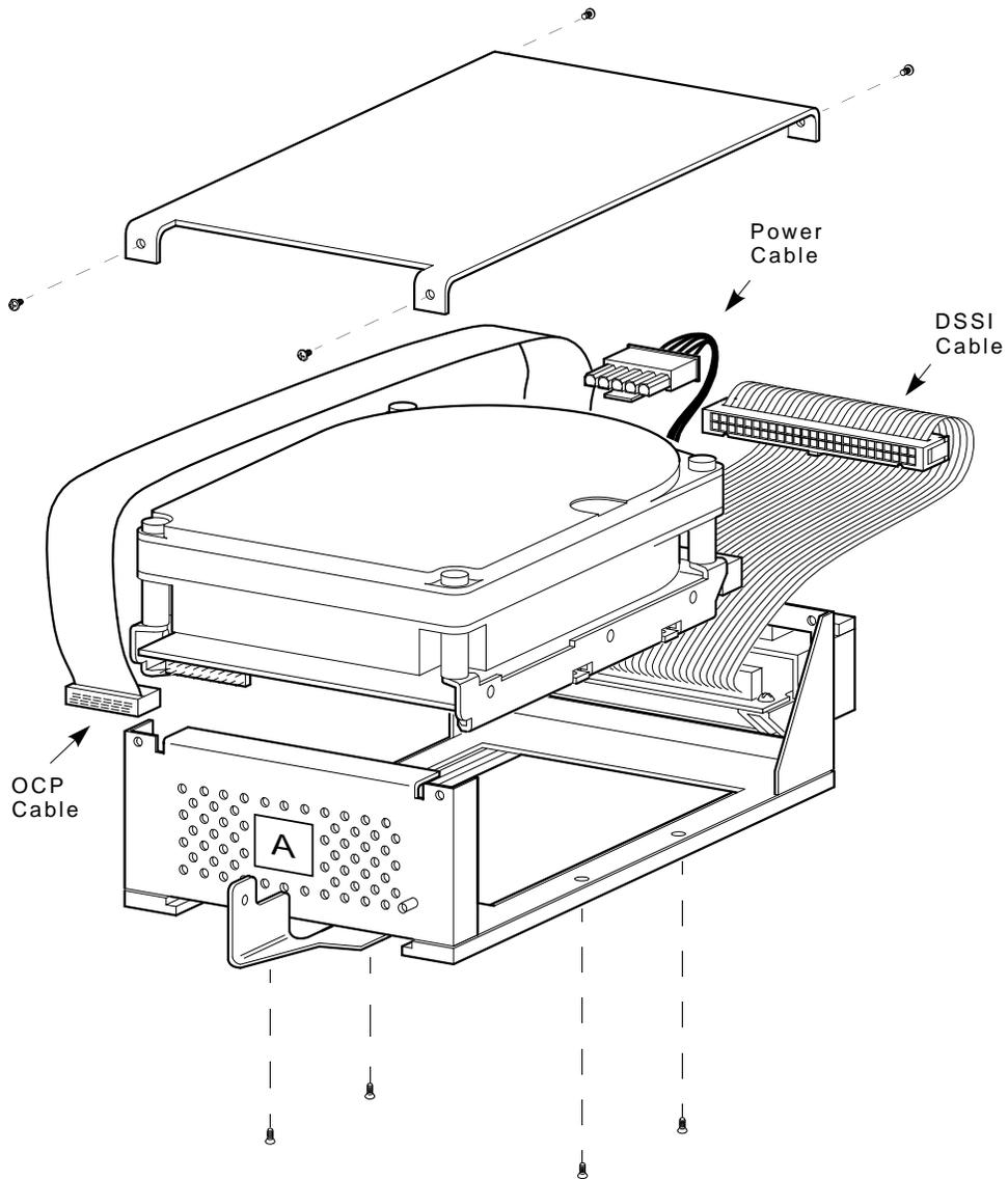
6. Remove the four screws holding the top cover on the carrier and remove the cover.
