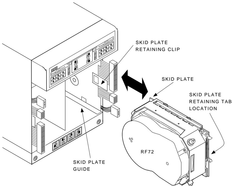
**Figure 6-4 Disk ISE Skid Plate and Wedges**
