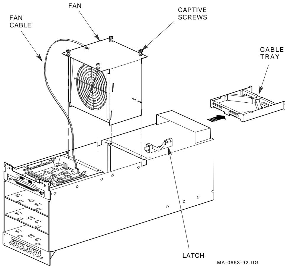
10. Orient the replacement fan assembly with the fan motor facing the front of the enclosure and with the fan cable exiting on the left top of the assembly.
