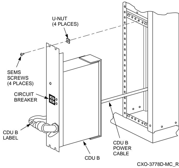
**Figure 6-4 Rear Power Cord Installation**
