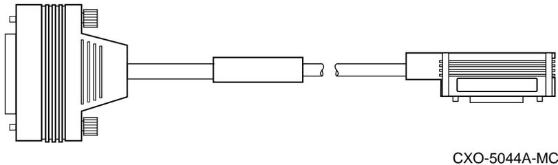
See Figure 3–24 for where to attach the straight end of the internal bus cable into the HS1AD device bus adapter port on the rear of the server processor. This server processor will only have the port labeled “FIRST HS1AD.”
