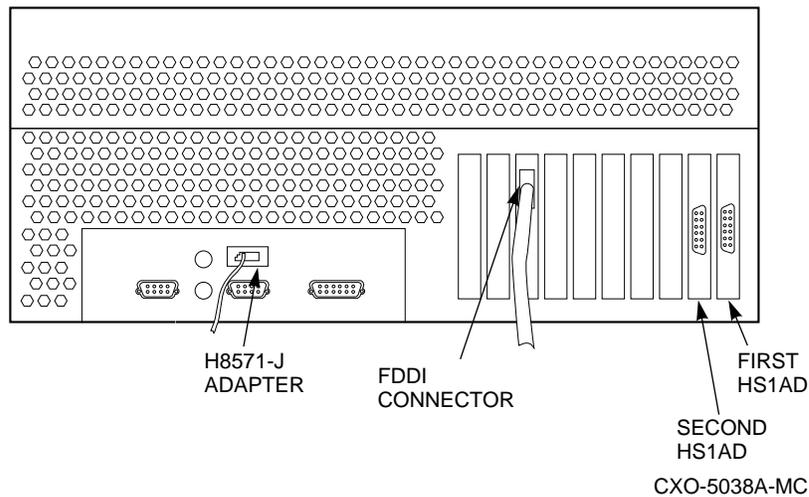
3. Connect the other end of the terminal cable to the EIA terminal port on the rear of the StorageWorks FDDI Server cabinet using an H8571–J adapter as shown in Figure 3–29.
