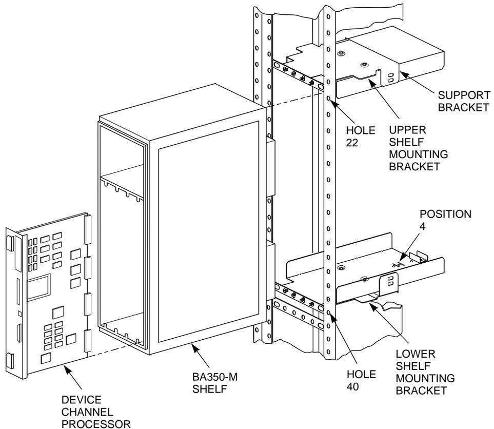
Figure 3–11 shows an exploded view of the components of the BA350–M shelf assembly:
