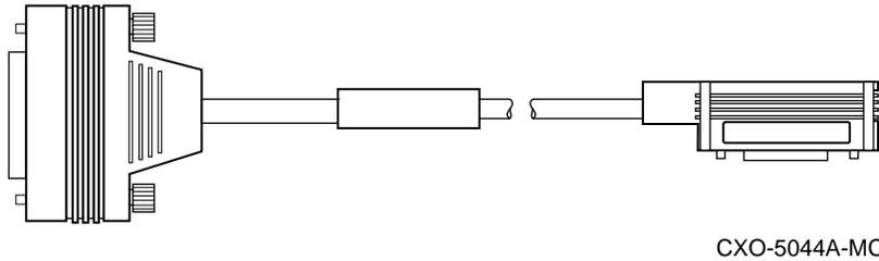
Use the right-angle end of the internal bus cable to attach to the HS1CP device channel processor trilink connector (refer to the connector on the *right* in Figure 9–9).
