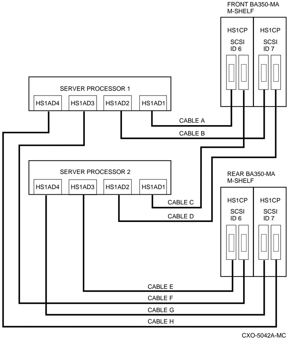
**Figure 9–8 Cabling Diagram for HS241/HS280**
