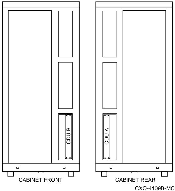
2. See Figure 6–2 to identify and locate CDU A. Identify the location for the installation of CDU B.
