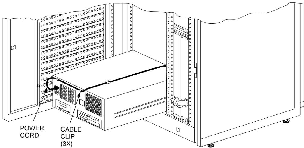
2. Attach three adhesive-backed cable clips to the new server processor. Two clips are attached to the front of the server processor; the third clip is attached to the top as shown in Figure 3–21. Two clips are attached to the front of the server processor; the third clip is attached to the top as shown in Figure 3–21.
