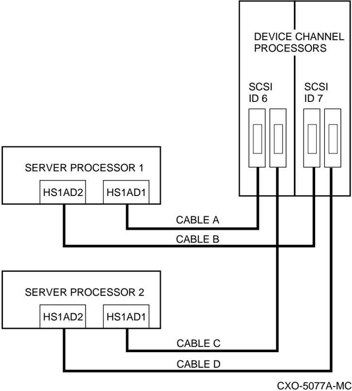
**Figure 7-4 Device Channel Processor Installation**
