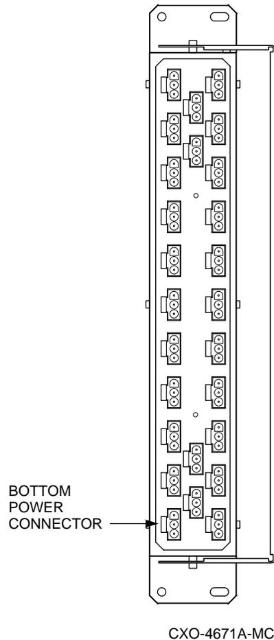
6. Install a new power cord to the bottom connector on the CDU. Route this new cord to the bottom front of the cabinet.
