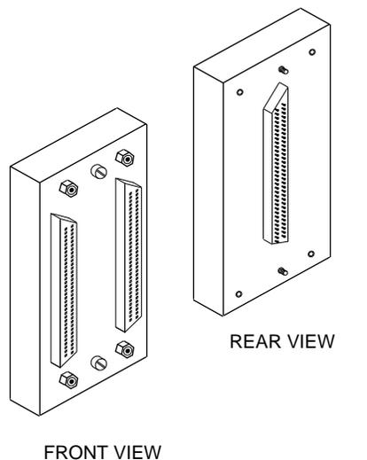
Be aware that the trilink connector block (Figure 9-6) is the interface between the HS1CP device channel processor and other internal bus cable connections. It is the *trilink* that you can disconnect and connect safely when you have a mating guide installed. In a power-on situation, you must work around any internal bus cable or terminator connections to the trilink *without* disconnecting them.
