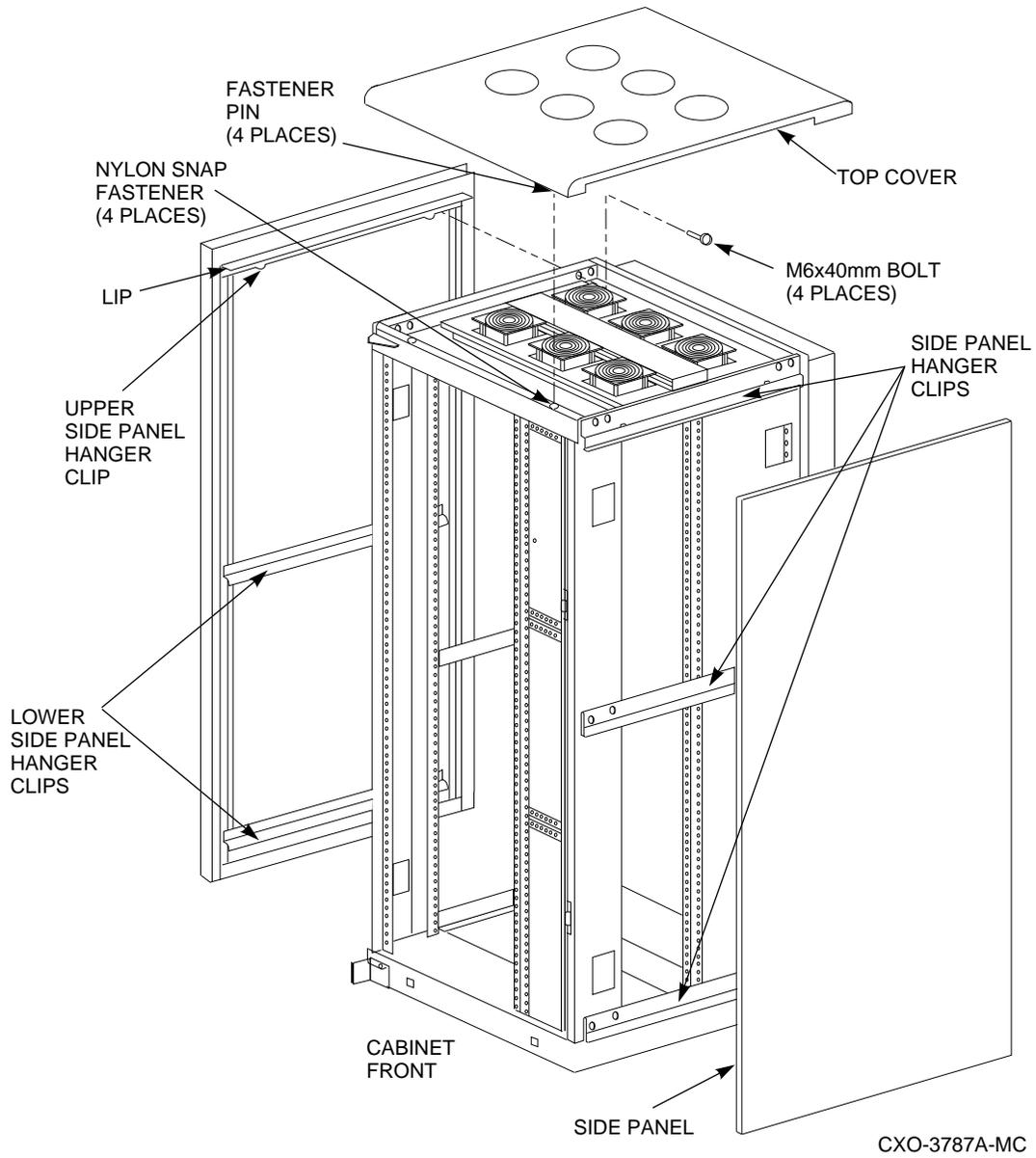
**Figure 3–2 Relocate ESD Bolt to Hole 19**
