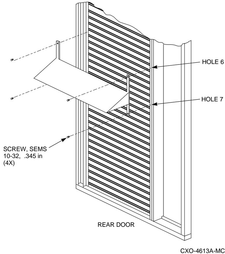
3. Install the horizontal air baffle to the rear door at hole positions 6 and 7 (from the top of the door) on both sides. Secure the baffle with 10-32 x .343 inch SEMS screws. When the rear door is closed, the horizontal baffle slides over the vertical air baffle (see Figure 3-7).
