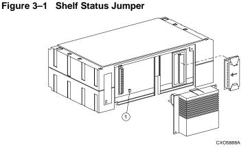
When the controller or adapter can process the SHELF\_OK signal, install jumper W1 to route the signal to the I/O module.
