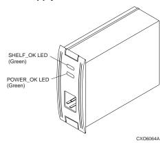
Figure 3–3 Power Supply Status LEDs
