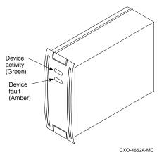
The upper LED (green) is the device activity LED, and is ON or FLASHING when the SBB is active. This is driven directly by the SBB storage device.
