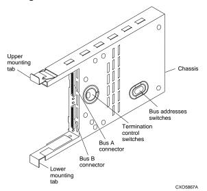
Figure 3–5 Single-Ended UltraSCSI I/O Module
