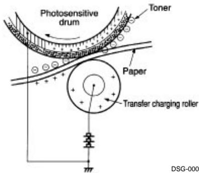
In the transfer process, the toner image is attracted from the OPC drum to the sheet of paper by the highly charged transfer charging roller. Like the primary charging roller, the transfer roller is made of a conductive foam rubber like compound.
