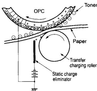
The transfer process leaves a powerful static charge that attracts the sheet to the OPC drum. The static charge eliminator reduces the charge, allowing the sheet to separate from the OPC drum. Malfunctions of the static charge eliminator produce the distinctive image defect that is described in Section 8.6
