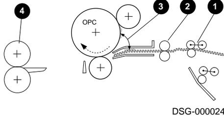
The *PRINT* signal from the controller board initiates a paper feed process. The cassette paper feed rollers ❶ or the refeed rollers move paper into the nip of the registration rollers ❷.
