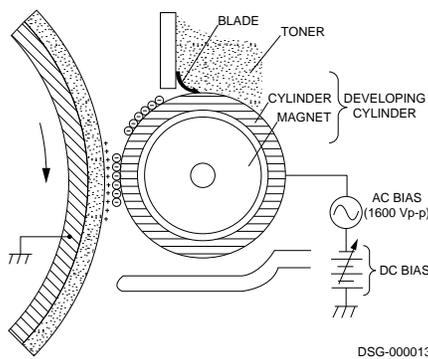
During the development process, the invisible latent image is painted with toner, producing a visible image on the surface of the OPC drum.
