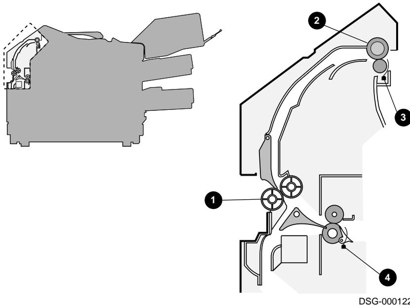
The active parts of the face-down paper path are the gate unit **1**, delivery rollers **2**, and fixing exit rollers. The rollers are gear driven by the main motor. When the top door is closed, the gear mounted on the top door meshes with the green drive gear to the left side of the fusing unit. Also, a tang on the top door presses a lever that meshes the right-side fusing unit gear to the main motor gear train.
