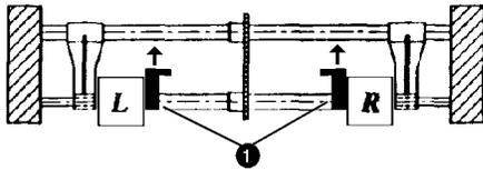
2. Remove both blue retaining **1** rings by pulling them in the direction shown.
