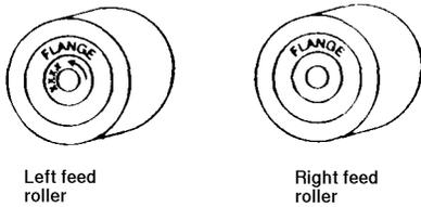
1. Locate the new left and right feed rollers according to the markings shown. The four X marks identify the left feed roller. The right roller has no such mark. Position the new feed rollers next to the LCIT.
