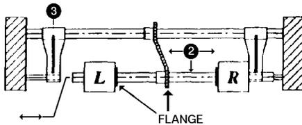
3. Slide the shaft **2** to the right to remove it from the left arm **3**.
