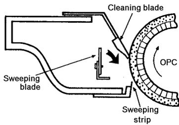
After the toner image is transferred and the sheet travels to the fusing unit, residual toner is cleaned from the OPC drum surface. The cleaning blade scrapes any remaining toner off the OPC drum. The sweeping strip gathers the toner and funnels it into the sweeping blade. The rotating sweeping blade moves the exhausted toner into a reservoir. The toner stays in the reservoir until the customer replaces and discards the EP-N cartridge.
