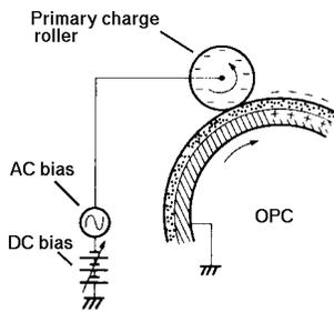
The primary charging roller distributes an even charge across the OPC drum. AC and DC biases charge the primary charging roller. The density adjustment potentiometer provides some adjustment for customers who like a darker print.
