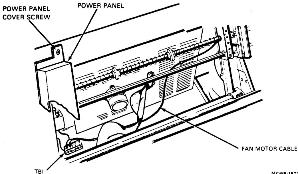
Figure 4-46 Blower Motor Cable Leads
