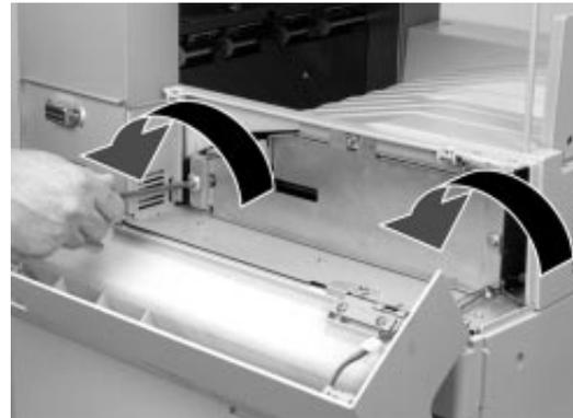
6. Loosen the two captive screws securing the grounding bracket and remove the bracket.
