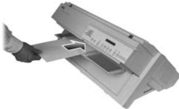
*Inserting the Cut Sheet*
