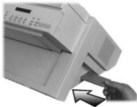
*Inserting the Set-Up Card*
