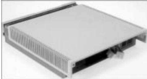
4. Remove the two screws holding the power supply to the system box frame.
