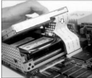
4. Remove the three screws holding the floppy disk drive in its frame, then slide the drive out of the frame.
