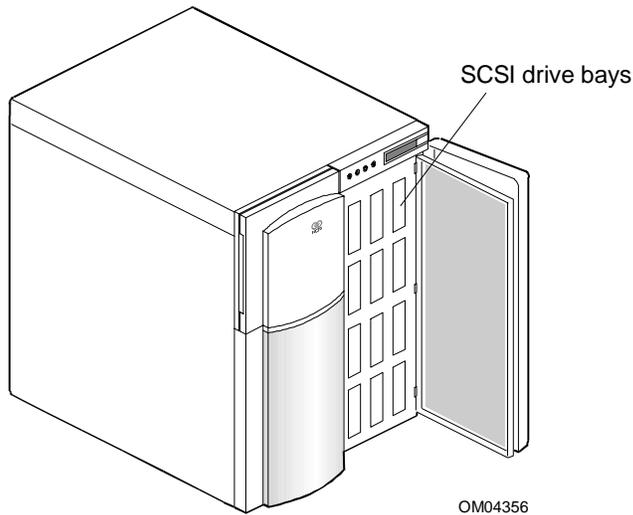
The right side of the system contains 12 bays for 3.5-inch SCSI-2 SCA hard drives and two hot-swap backplanes. Each backplane supports six drives. The backplanes require an 80-pin SCA connector on the drives you install.
