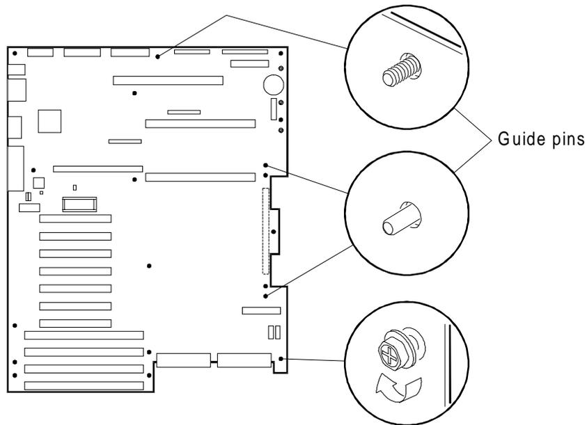
7. Align the primary system board intermodule connector with the secondary system board intermodule connector. Seat the board in the chassis and connect the intermodule connectors.
