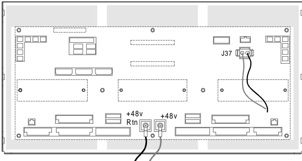
5. Unplug the cable from J37 (two-pin mate and lock connector) on the power distribution backplane.
