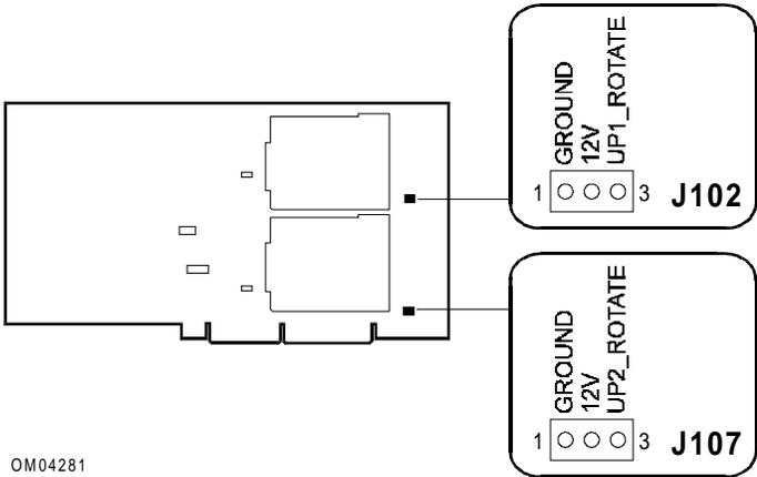
J102 and J107 are connectors to power optional fan sinks to cool the processors while the board set is being tested outside of the chassis on a test bench. Each fan sink comes with a 3-pin connector wire. The connectors are not used in normal system operation.
