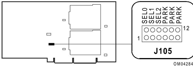
**CAUTION:** Damage to the processor can occur if you select a jumper setting frequency that is greater than the actual frequency of the processor.
