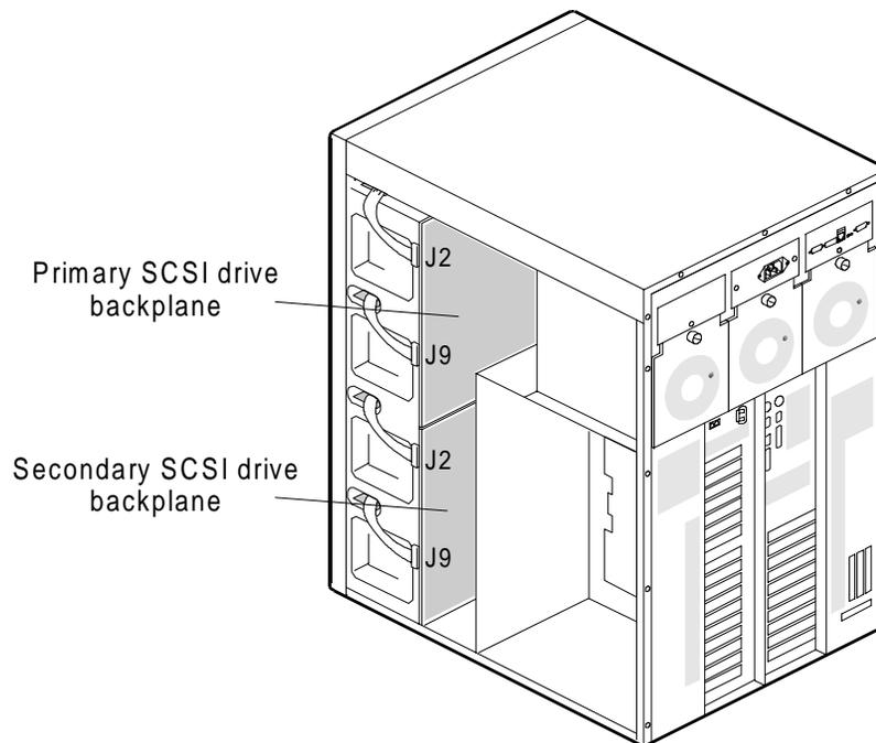
4. Carefully remove the fan assemblies on this side from the chassis. Do not let the inner fan fall out of the fan assembly.
