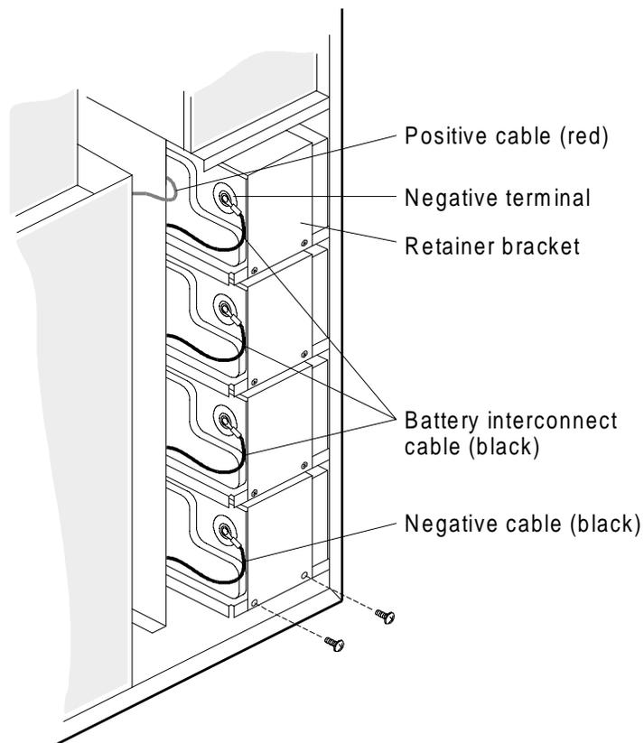
3. Disconnect the negative cable (black) from the bottom battery negative terminal. Use either a #6 or #8 metric or socket wrench, depending on the size of the nut.
