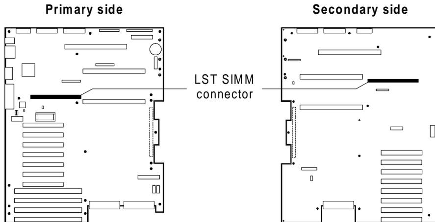
6. Open the retaining clips. Carefully pull the LST SIMM out and up at a 45-degree angle.
