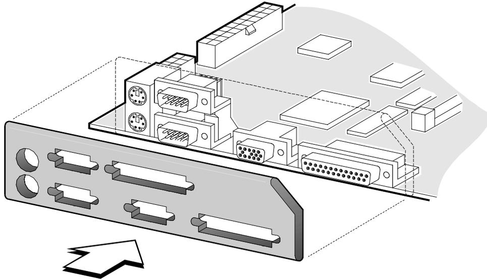
5. Position the board with the I/O connectors toward the chassis back panel. Slide the board toward the back of the system until the I/O connectors protrude through the openings in the back panel.
