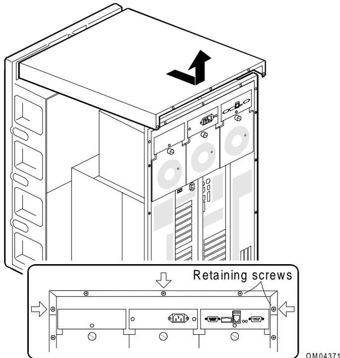
**Important:** Remove side covers first. You must remove both side covers before you can remove the top cover.
