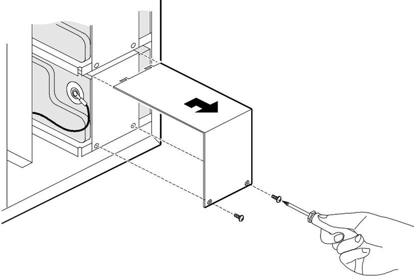
6. Repeat Steps 4 and 5 to remove the three remaining retainer brackets.
