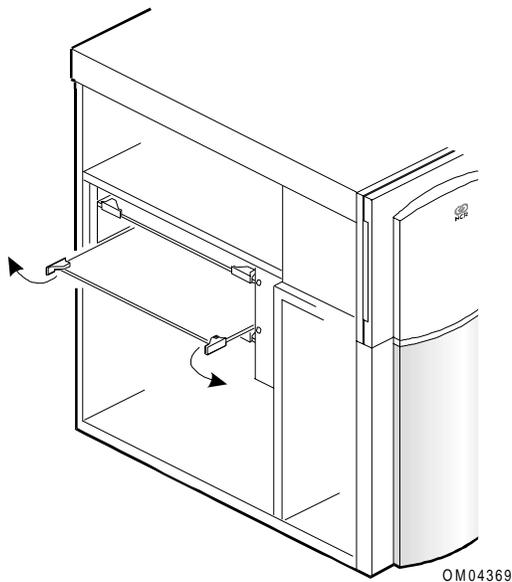
5. Holding the board by the corners where the handles are, carefully pull it out until the edge connectors are free from the system board connector.
