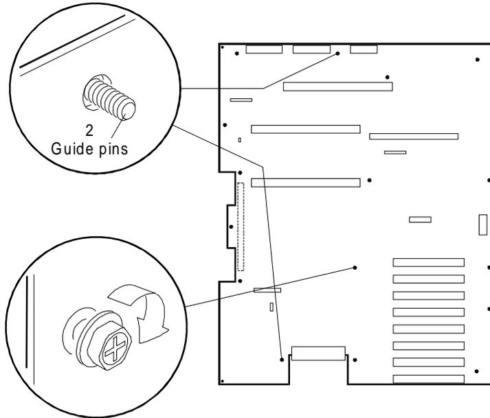
5. Align the secondary system board intermodule connector with the primary system board intermodule connector. Seat the board in the chassis and connect the intermodule connectors.
