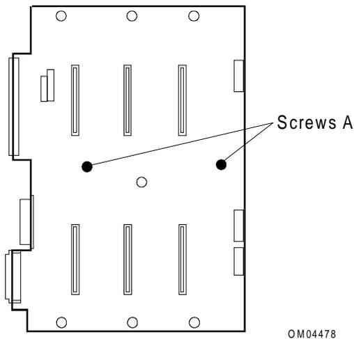
4. Reconnect all cables to the backplane. The SCSI signal cables have precise folds that are intended to help the cables fit in the space allowed and to correctly orient the pin 1 side of the cable(s) (red stripe).
