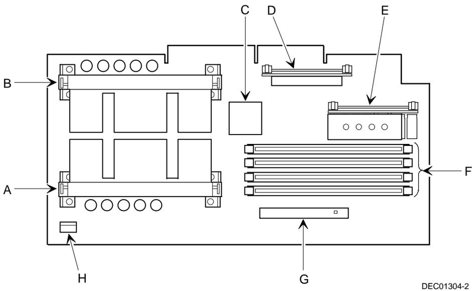
Figure 3-5. Pentium® II Processor Module Component Locations
