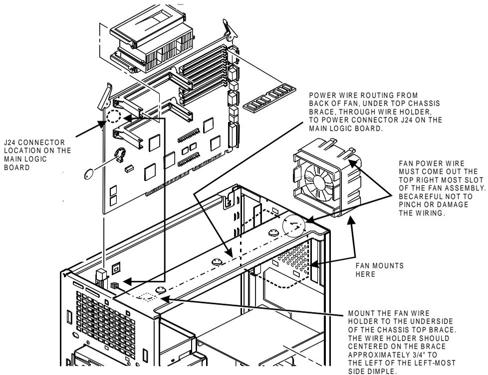
**Figure 1-11. Wiring Path for additional Fan Assembly**
