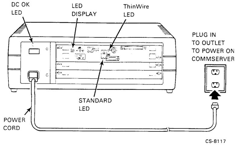
Figure 4-6: Initial Power-Up of the DEC Commserver 150
