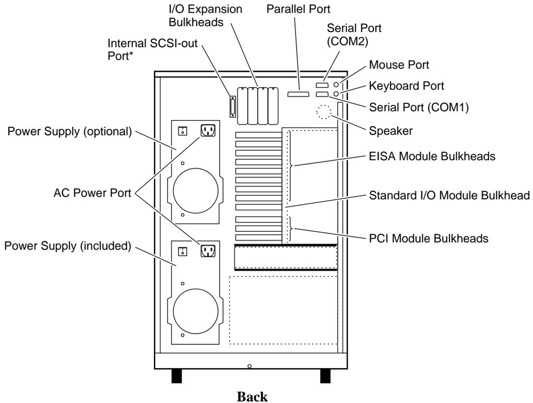
\* If not used, internal SCSI-out port must be terminated with External Terminator (12-37004-04) included with system.
