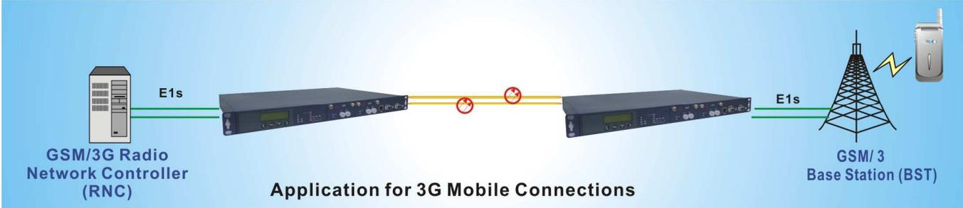
Figure 2-1 Terminal Multiplexer (TM) application
