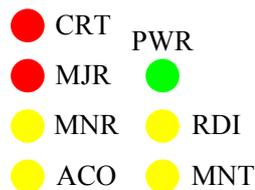
Figure 3-3 Alarm indication LED
