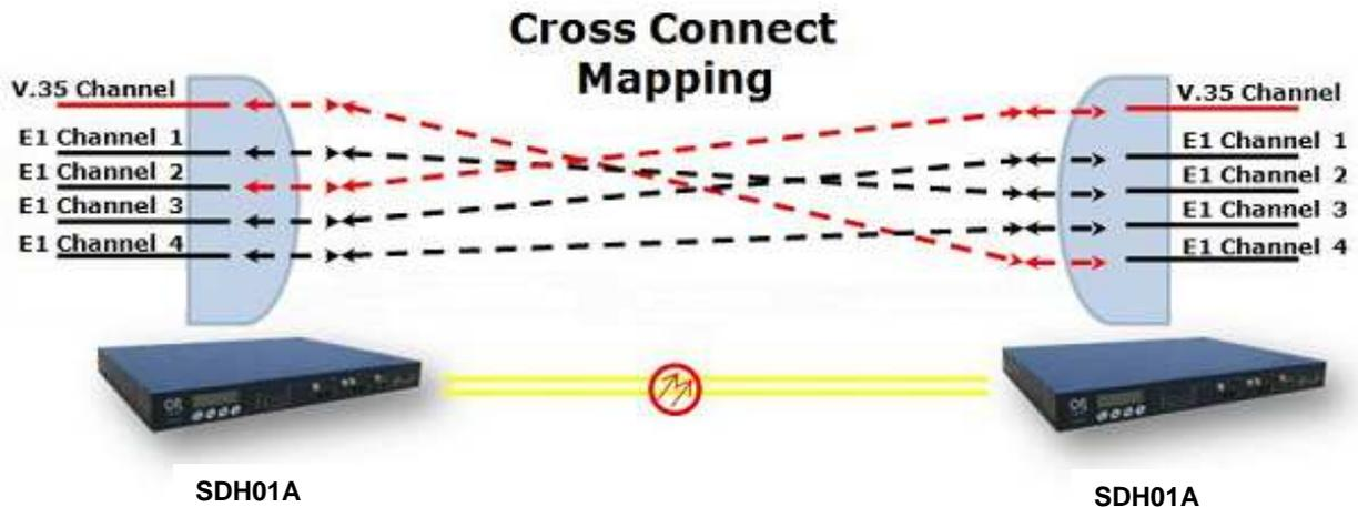
Figure 2-4 Cross Connect Mapping
