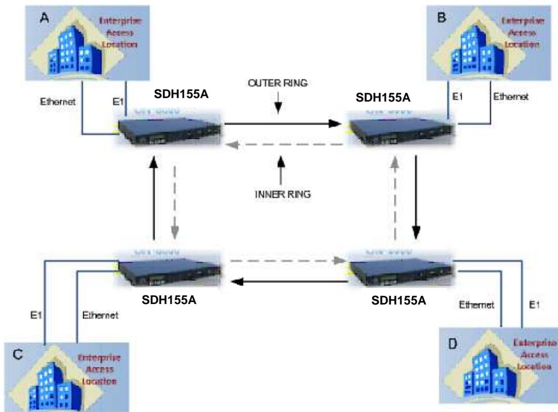
Figure 2-5 EoS (Ethernet over SDH) ring protection scheme
