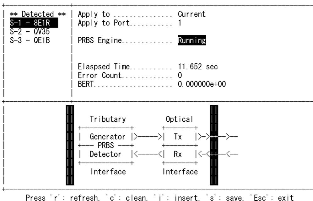
The above example illustrates the BER test on Slot 1 Port 1, an E1 channel.
