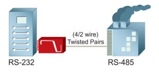
The ic485-3 Interface Converter provides conversion between RS-232 interface and RS-485 standard interface. The RS-232 interface connection is via the unit's DB-25F female D-Type connector, while the RS-485 side's connection is via a five screw terminal block.
