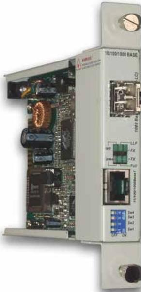
The model shown has an industry standard SFP with LC. The converter is also available with GBIC or fixed transceiver.
