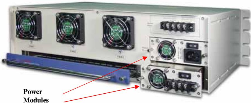
Figure 2-5 Power Modules for **FRM301**
