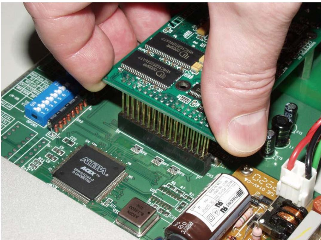
Figure 2-4: Align the header pins to PCB header.
