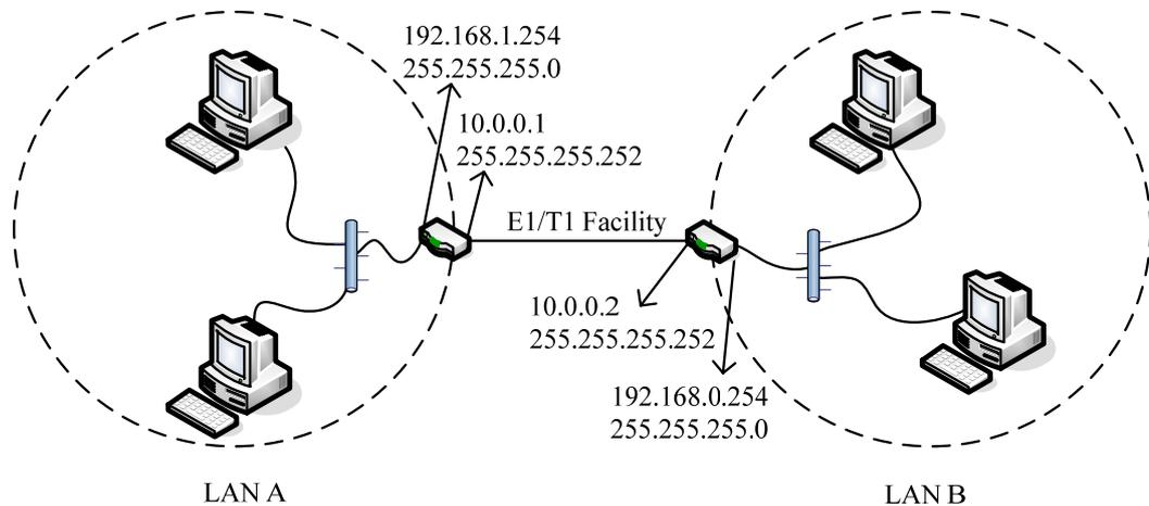
Figure 3-6 ET100R Point-to-Point Application and RIP implementation
