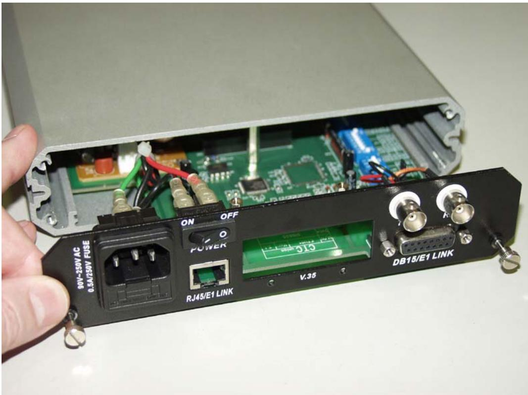
Figure 2-2: Open ETU/TTU Series Unit
