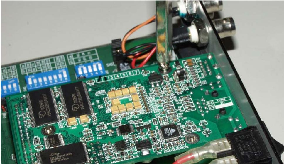
Figure 2-5: Secure the module with three supplied screws.
