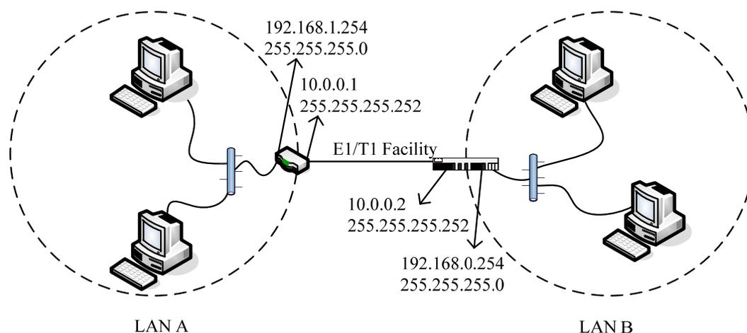
Figure 3-2: ET100R Point-to-Point Application with Cisco router
