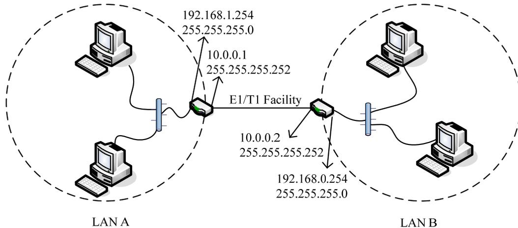
Figure 3-3 ET100R Point-to-Point Application example
